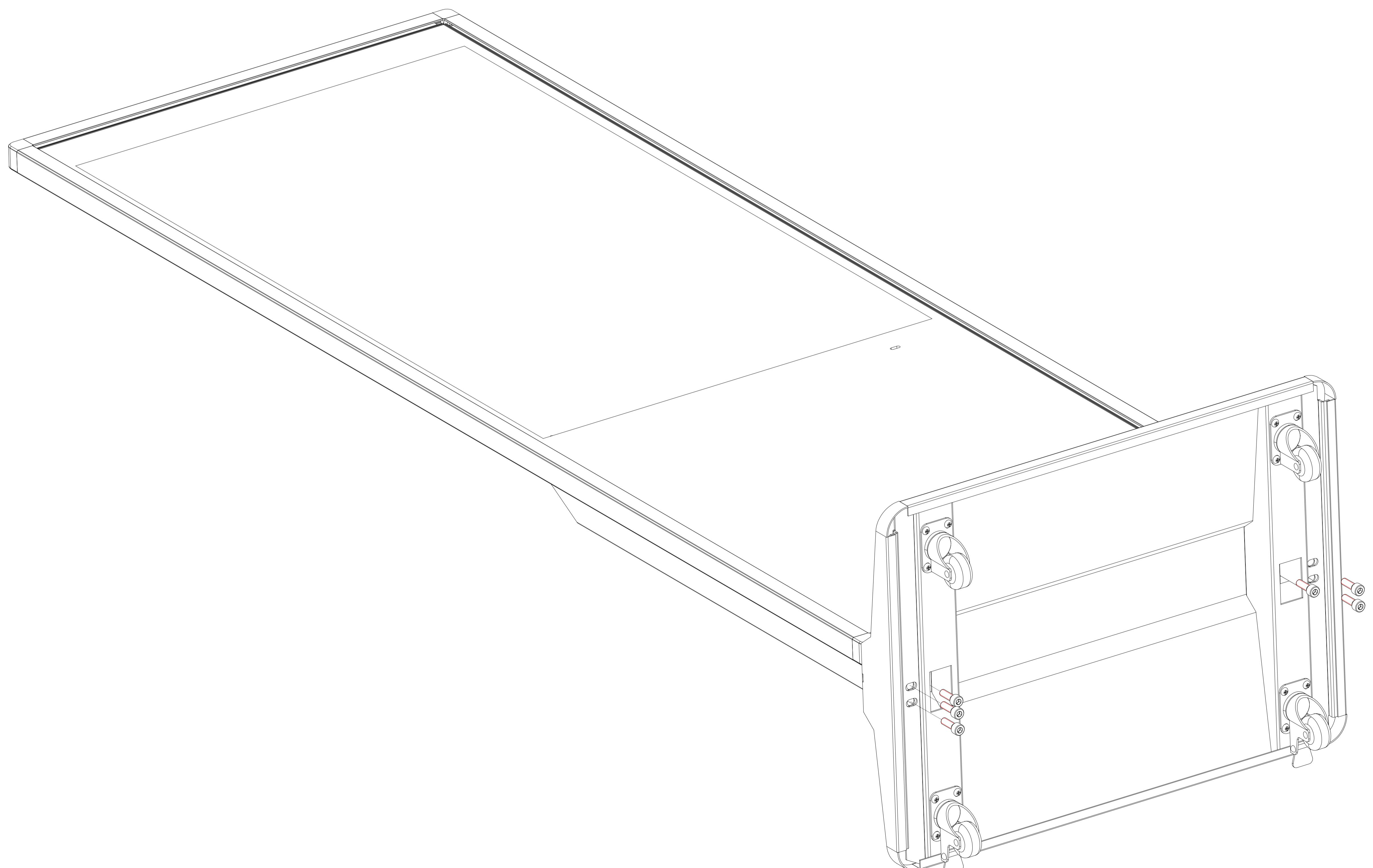
Place the device on a flat surface and insert it into the corresponding notch in the base.
