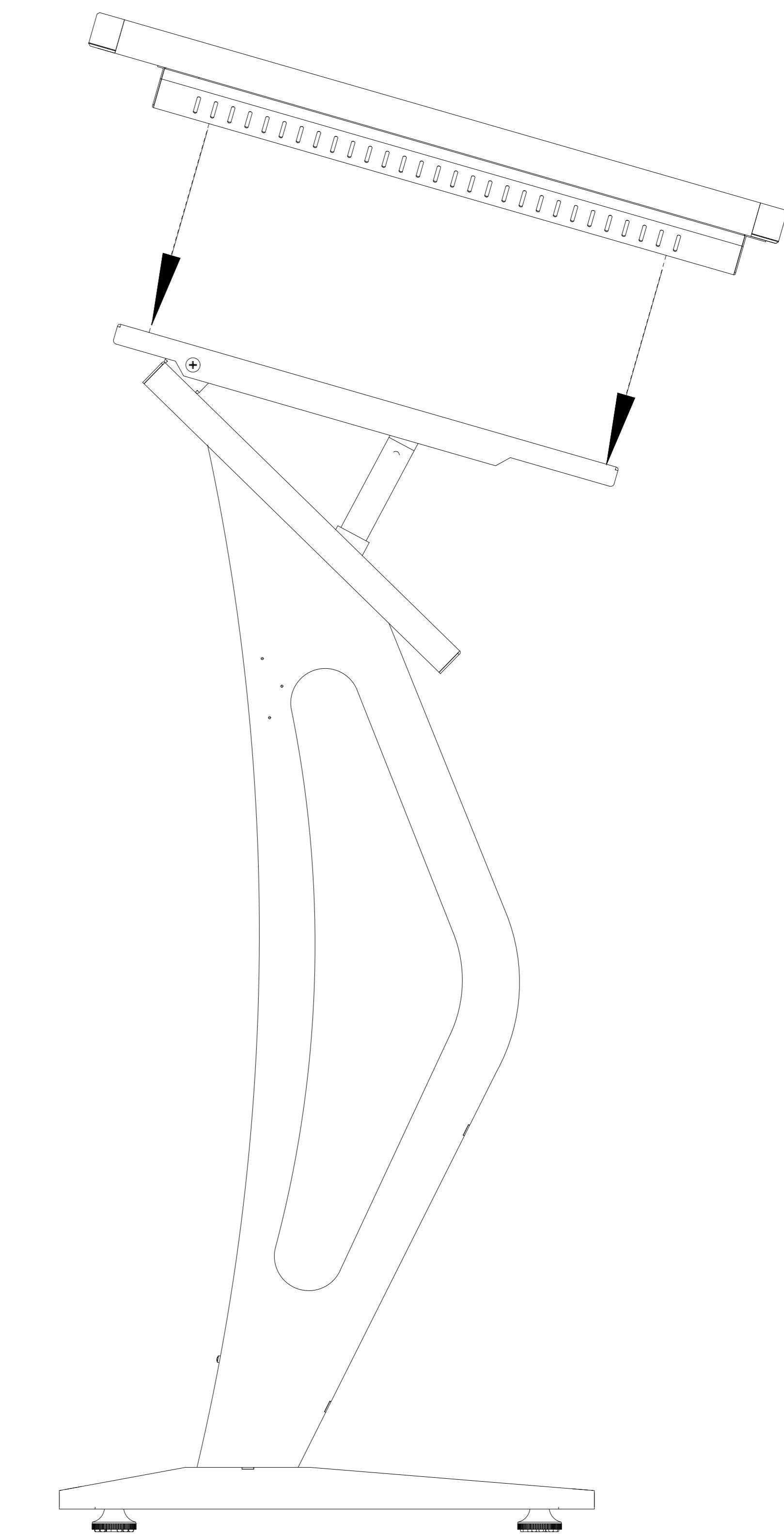
1. Screw the screws into the wall-mounting holes on the back cover of the machine, leaving a step for the mounting plate.
