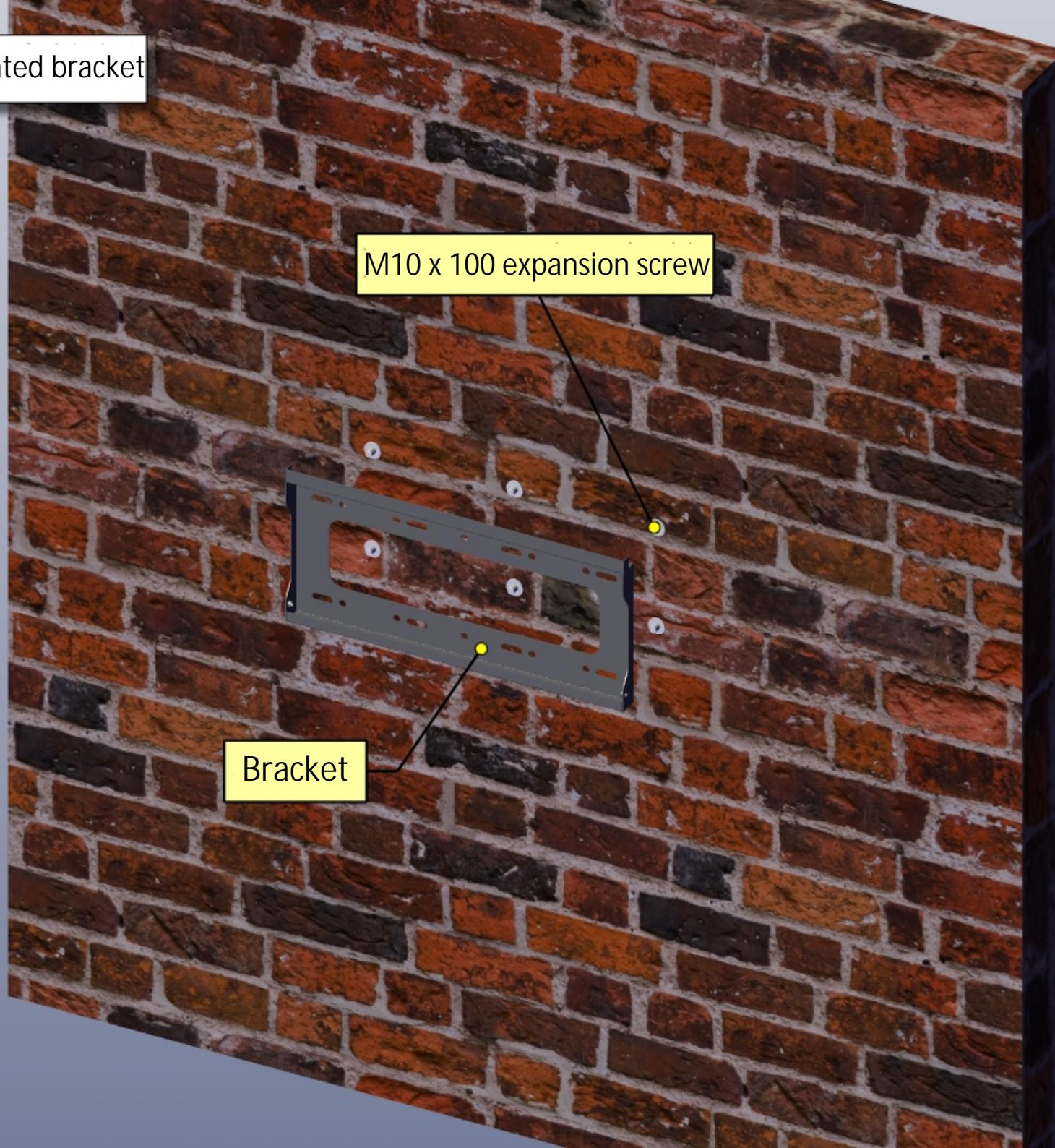
6. Align the wall-mounted bracket with the expansion bolts and tighten the nuts
