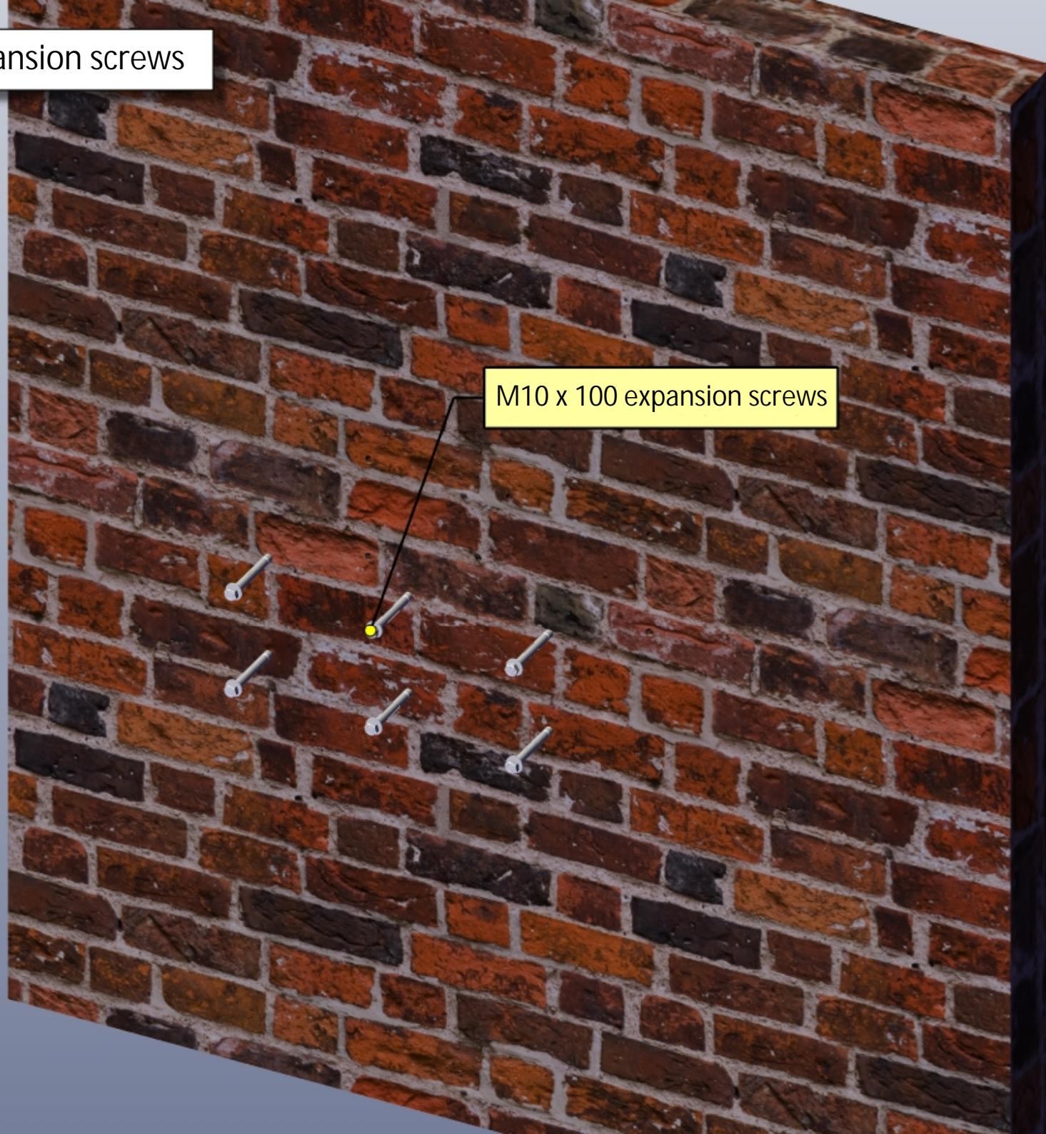
4. After installing the expansion screw, remove the nuts
