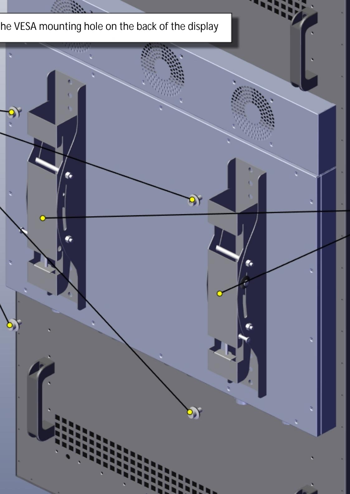
8. Hook assembly and display installation complete
