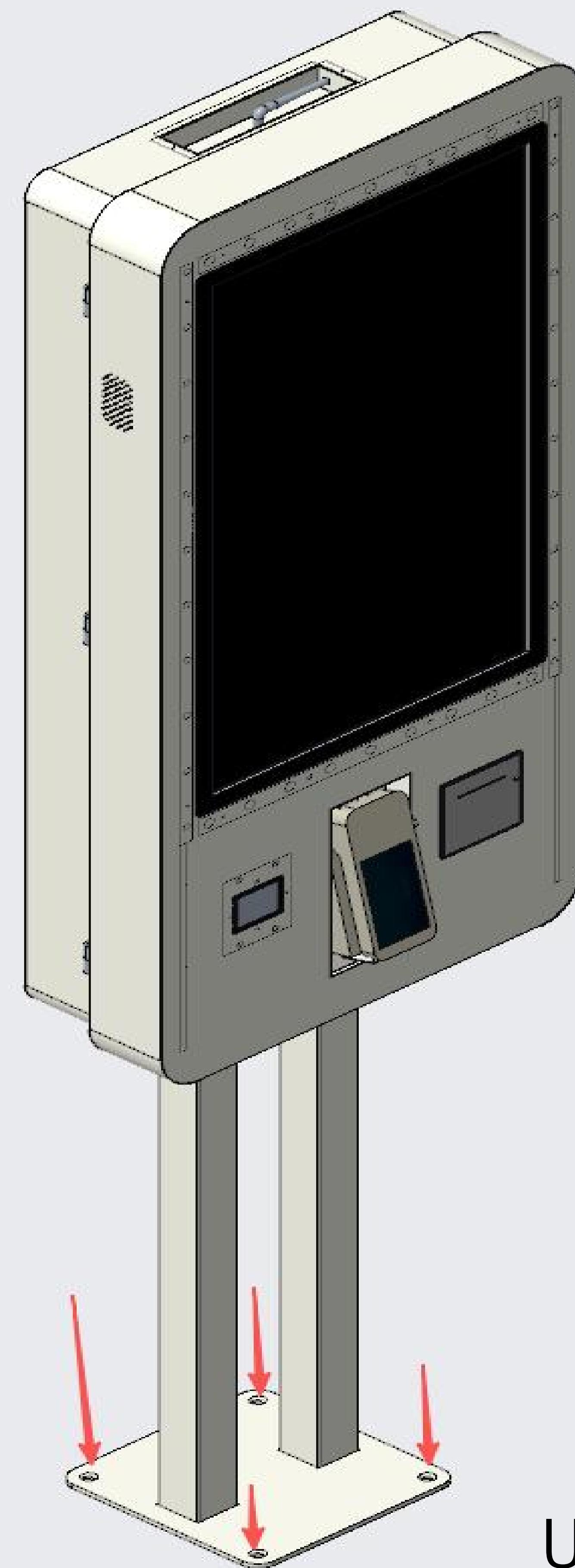
Use expansion screws to secure the stand to the floor
