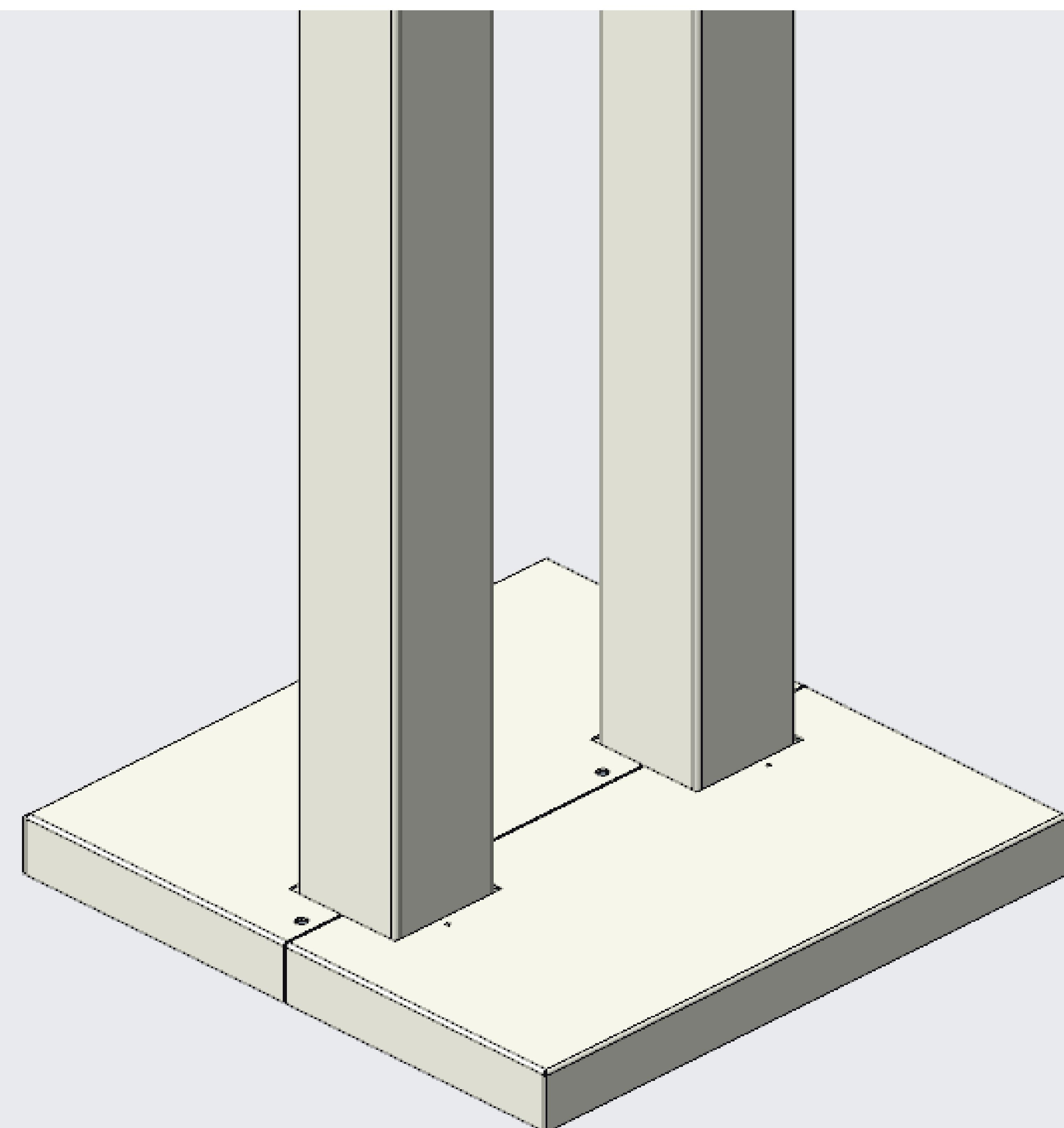
Finally, place the cover on the stand to hide the expansion screws
