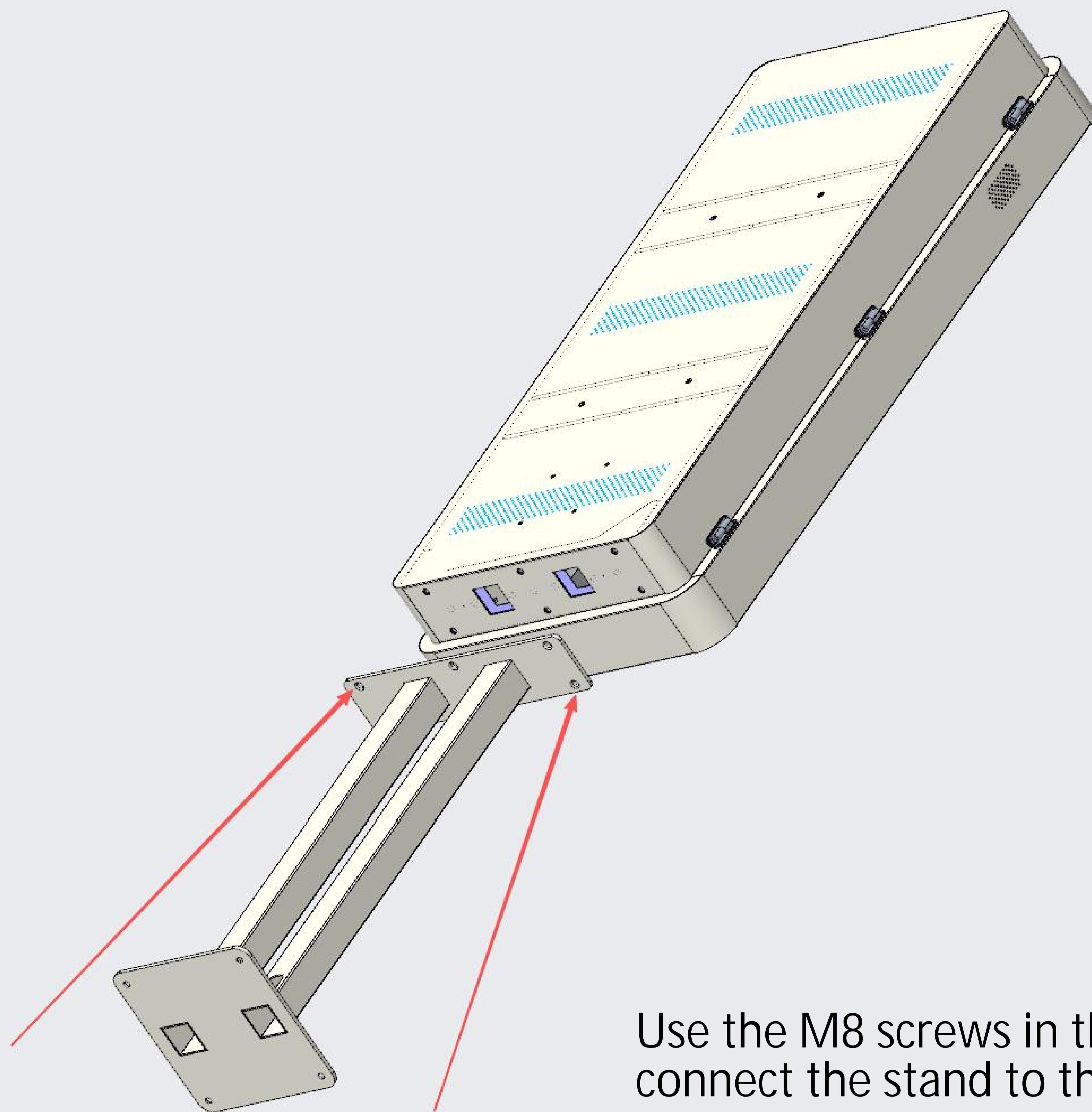
Use the M8 screws in the accessory kit to connect the stand to the device
