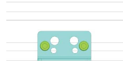
Move the angle iron with the screws fixed along the groove of the bracket to the designated position and tighten the screws
