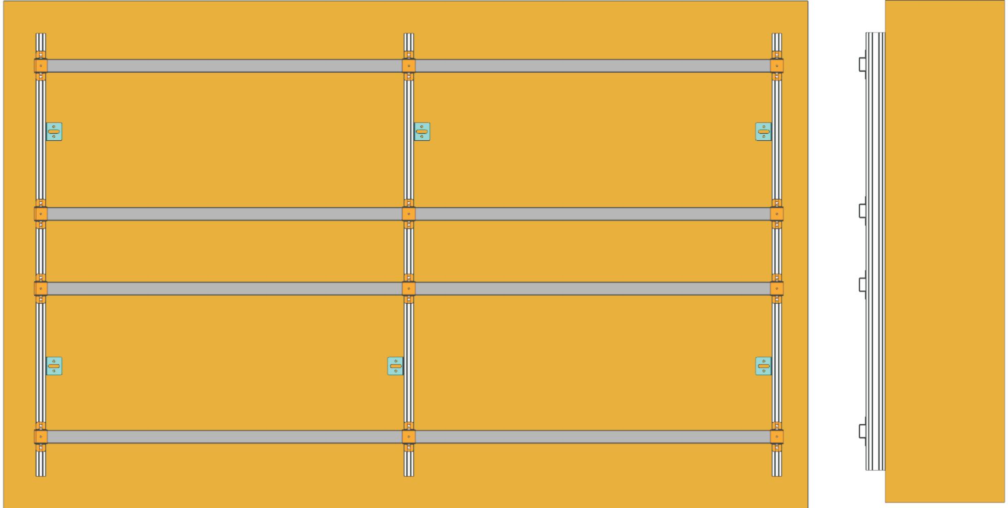
Attach the assembled bracket to the wall to be installed, mark the angle iron position and drill holes
