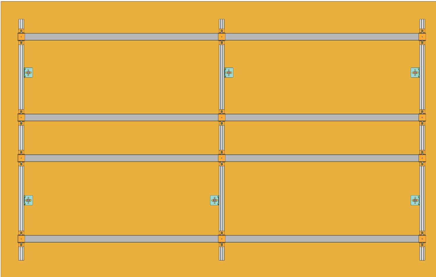
Stick the assembled bracket to the wall, drive the expansion screws into the wall, and tighten the expansion screws with a wrench
