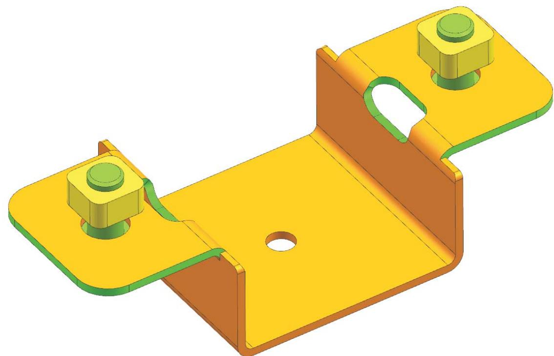
As shown in the figure, fix the M6 screws and nuts to the connector
