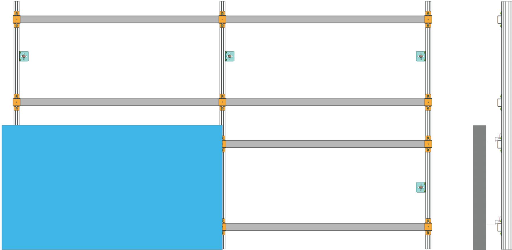
Connect the necessary cables, then arrange the screens from bottom to top, and use the adjustment screws on the hooks to adjust the screens to the correct position
