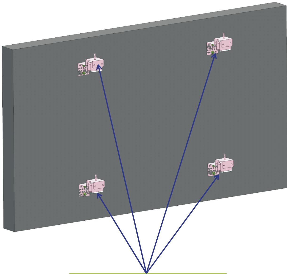
Use screws to fix the hooks at the designated positions behind the screen (4 hooks per screen)
